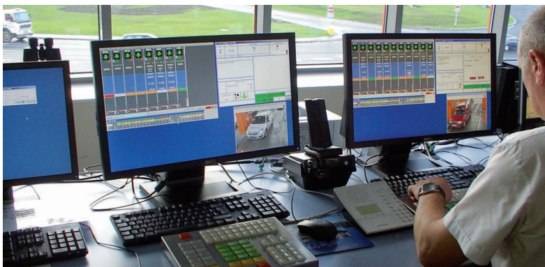
Only one operator for supervision and remote assistance of many plazas and dozens of automatic lanes.
