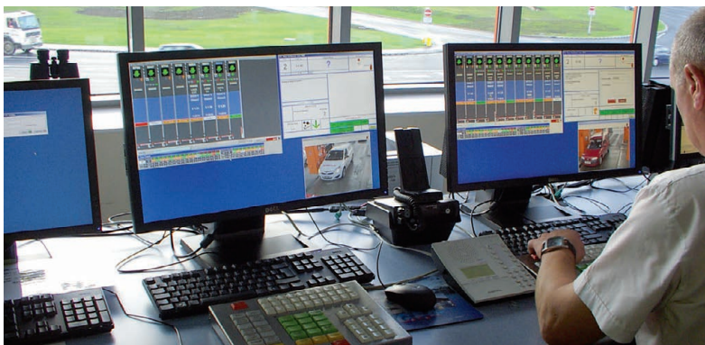
Only one operator for supervision and remote assistance of many plazas and dozens of automatics lanes.
